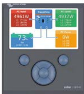
Color Control GX, showing a PV application
